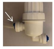
Take the remainder of the hose spool. This section of hose will be running from the outlet side of the strainer to the dry bilge unit. Make sure the tip if the hose is cut evenly. If it is not, cut it again with a scissor to make it even. Then insert the hose firmly into the guick connect
